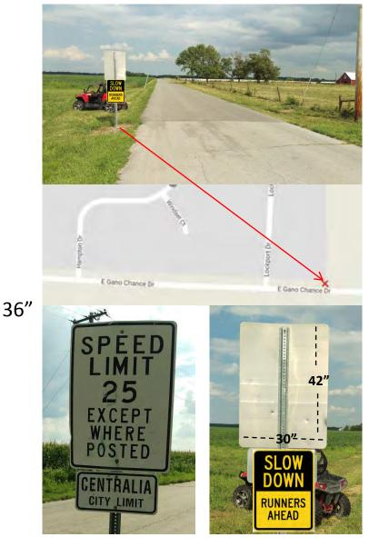
I propose mounting the "Runners Ahead" sign on the back of the existing sign at the City Limit on East Gano Chance. I would have the sign made from aluminum with a stainless steel hinge and latch so they may be "opened" during practice and then closed once practice is over. The sign would be removed after the season is complete. Thanks in advance for your consideration and advice.
